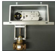
Construction: The enclosure is constructed of sturdy marine grade aluminum .080-inch (2 millimeters) thick. Any seams are continuously welded and ground smooth, and a corrosion resistant coating is applied to the entire enclosure for an extra degree of protection. The cover is secured with two quick release latches which allow easy access for maintenance.
