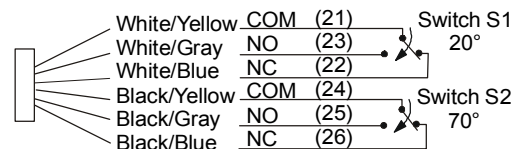
Figure 9: Wiring Diagrams for ES53 Models
